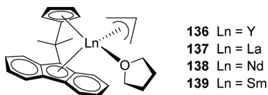
Fig. 13. Allyl ansa -lanthanidocene single-component catalysts used for syndiospecific styrene polymerization [162,163].
